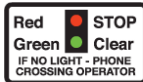
Miniature warning lights at level crossing
